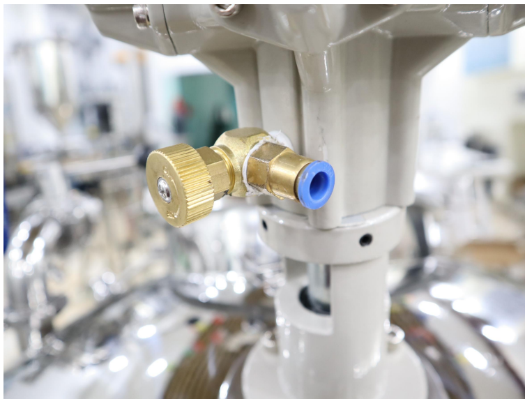
Gas inlet connects with the air compressor
